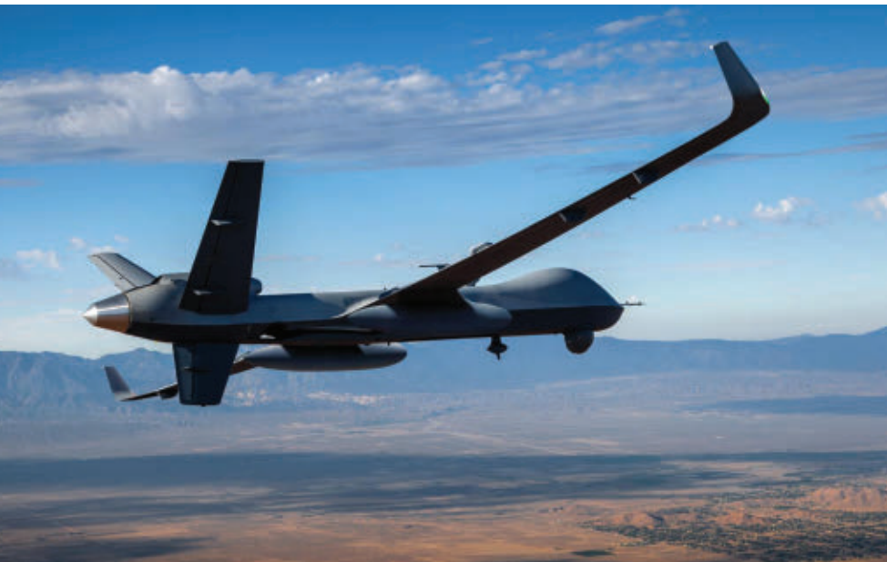
General Atomics Aeronautical Systems MQ-9B SkyGuardian version of its Predator UAV can provide persistent surveillance by flying in excess of 35 hours with air speeds to 210 knots at altitudes of more than 40,000 feet.
