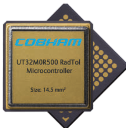
Cobham is offering the RadTolerant Arm Cortex -M0+ microcontroller for space applications with an integrated analog front end and on-board volatile and non-volatile memory.
