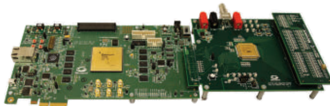
Microsemi integrates the company’s radiation-tolerant RTG4 field-programmable gate array on a variety of embedded computing boards for on-orbit space uses.
